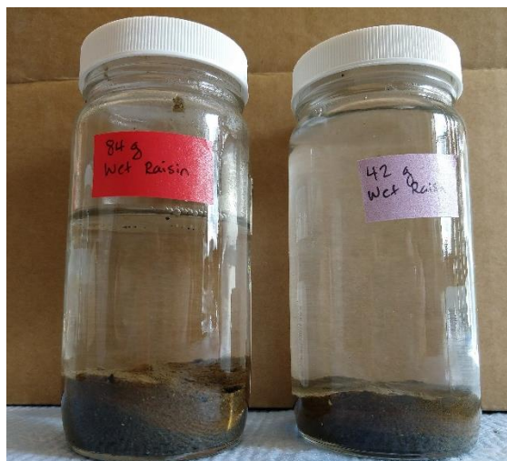
Figure 2: Modified OECD 308 Septa jar design. Wet Raisin substrate (84 g and 42 g) added to each jar with 1week incubation at room temperature in 10x diluted OECD 203 solution.
